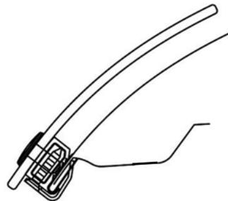
12. Insert a #6 x 5/8" screw through the 'L'-bracket and into the clip body.
