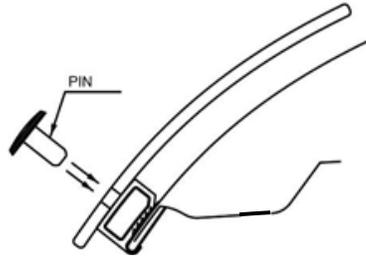
10. Place a clip body over the anti-abrasion film pads.
