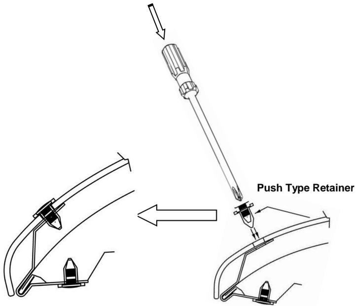
7. Place the deflector on the hood, resting on the four (4) metal brackets; align the holes in the deflector with the holes in the metal brackets. Insert a "push type retainer" through the hole in the protector, and into the bracket. Ensure the protector is well seated against the surface of the metal bracket, and push the center pin of the retainer assembly to lock it into place.
