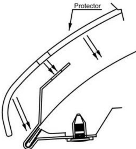
6. Place the deflector onto the metal brackets aligning the holes in the deflector with the holes in the metal brackets.
