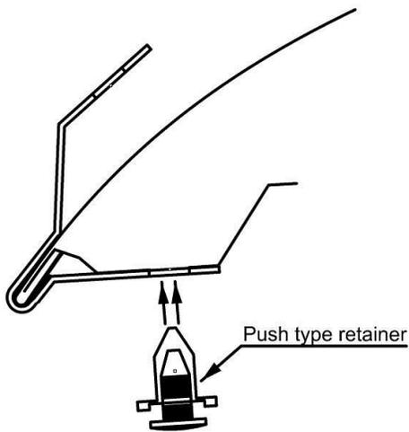
5. Insert a push type retainer through the metal bracket and into the hood. Ensure leg of the bracket is well seated against the surface of the hood and push the center pin of the retainer assembly to lock it into place. See *Illustration*.
