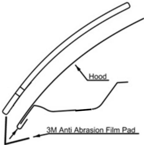
9. Peel and fold an anti-abrasion film pad in half over the edge of the hood in alignment with the remaining holes in the deflector.
