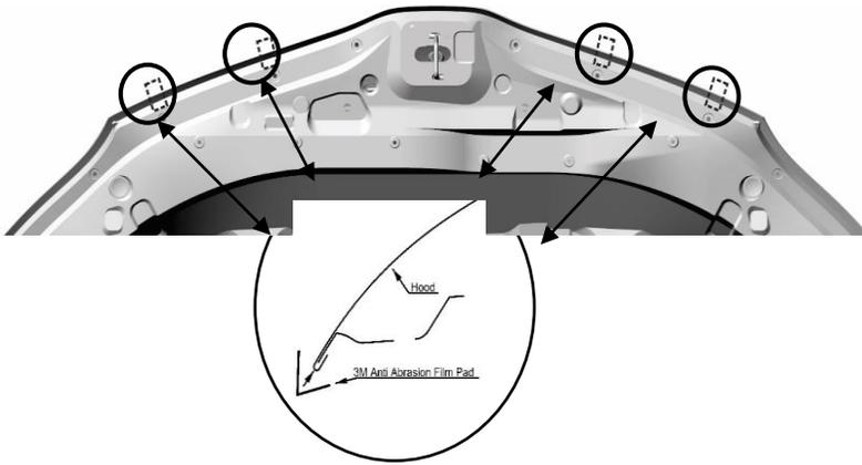
3. Open the hood of the vehicle. Peel and fold anti-abrasion film pads in half over the edge of the hood, in the four (4) locations shown.
