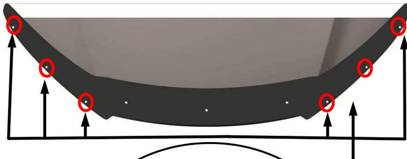
8. Peel and fold an anti-abrasion pad in half over the edge of the hood in alignment with the holes in the protector at the six locations over the headlights.
