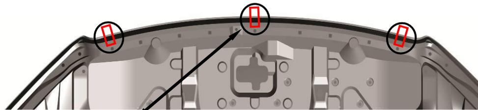
3. Open the hood of the vehicle. Peel and fold an anti-abrasion pad in half over the edge of the hood, in the locations shown.
