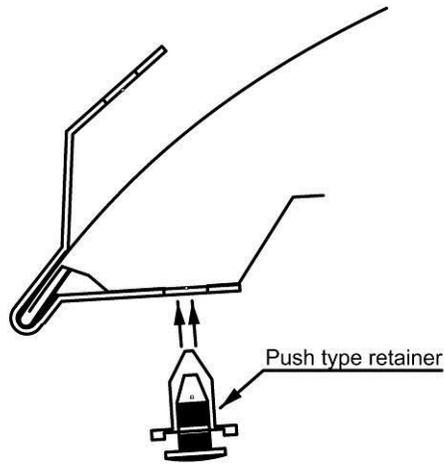
5. Insert a push-type retainer through the metal bracket and into the round hole in the hood. Push the center pin of the retainer assembly to lock it into place. See *Illustration*.
