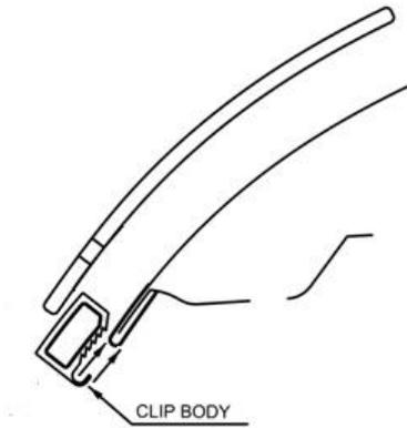
9. Place a clip body over each of the anti-abrasion pads on the edge of the hood.
