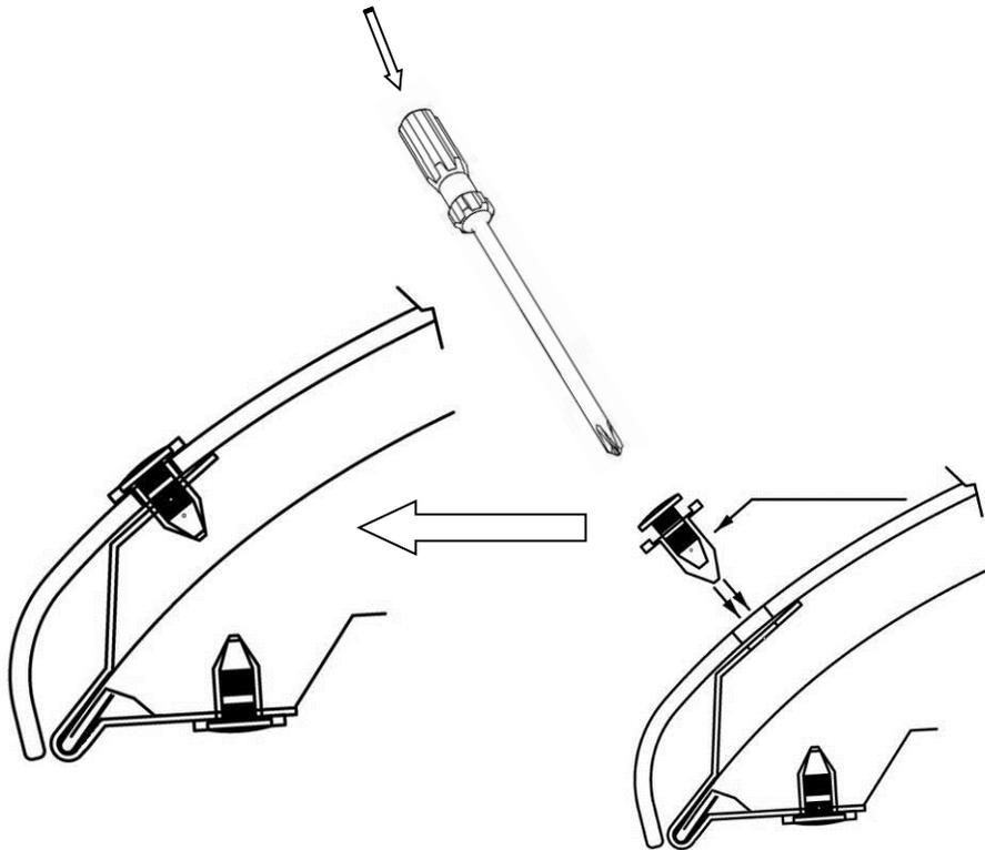
7. Align the 3 centre holes in the protector with the three (3) metal brackets
