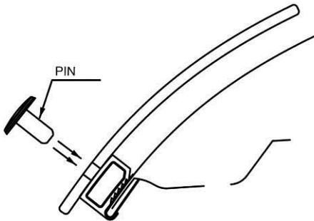
10. Insert a pin through the protector into each of the clips.
