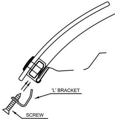
11. Insert a screw through an 'L'- bracket and into each clip.
