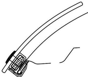
12. Make sure all the components are well seated together; the protector is centered on the hood, and then tighten the screws into the clips.
