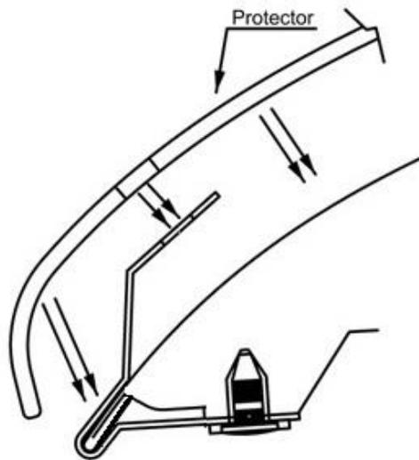
6. Place the protector onto the metal brackets.
