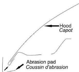
4. Locate the two small holes on the front edge of the protector and wrap a large abrasion pad around the hood edge at these locations. On some applications it may be easier to stick the abrasion pad to the underside of the hood at the appropriate locations and then pick up the hood protector to wrap the abrasion pad around to the top surface of the hood.
