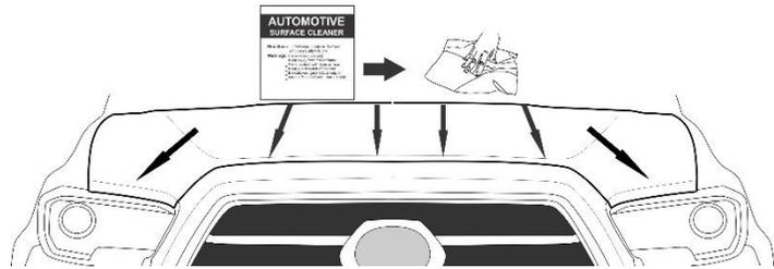
1. Use the surface wipe provided and wipe down the area (approximately 15cm (6 in.) from the hood edge) where the hood protector will be installed. Wipe dry with a soft cloth or paper towel. This will remove any wax or grease and will ensure a cleaner surface for the adhesive to bond to. Return the wipe to its packaging for use in step 10.
