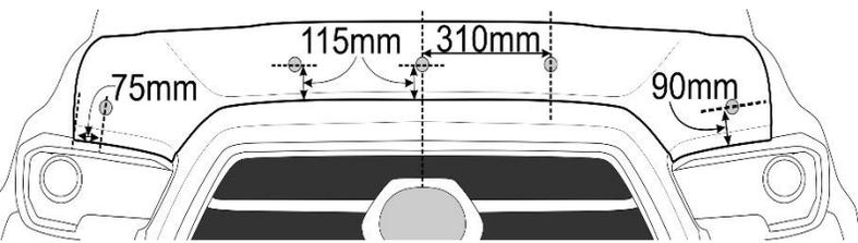
2. Place bumpers in locations shown in the illustration. Note that bumpers must be placed on the hood, not the hood protector. If they are placed on the hood protector, they will wear through the paint on your hood!
