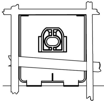
10. Remove the hood protector, and outline the perimeter of the pedestals with masking tape to help final installation.
