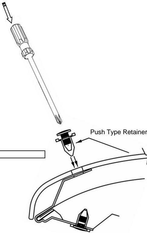
14. Place the hood protector on the hood resting on the four (4) metal brackets; align the 4 center holes in the protector with the holes in the metal brackets. Insert a “push type retainer” through the hole in the protector, and into the bracket. Ensure the protector is well seated against the surface of the metal bracket, and push the center pin of the retainer assembly to lock it into place.
