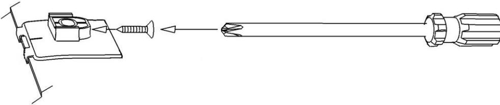
13. Start a #6 x 5/8 flat head screw into each pedestal a few turns. The tip of the screw must not protrude into the hole where the attachment pin will install later.
