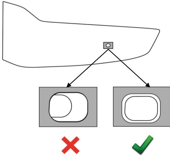
9. Confirm correct positioning of the pedestals, by adjusting the pedestal position on the hood to align with the holes in the hood protector.
