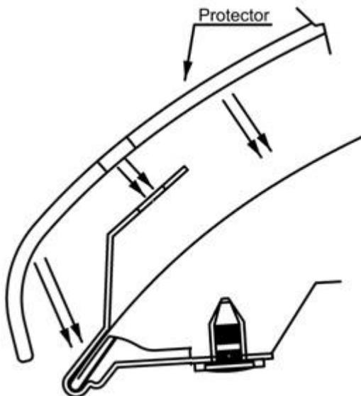
8. Place the protector temporarily onto the metal brackets aligning the holes in the protector with the holes in the metal brackets. This step will allow you to confirm the position of the adhesive pedestals.
