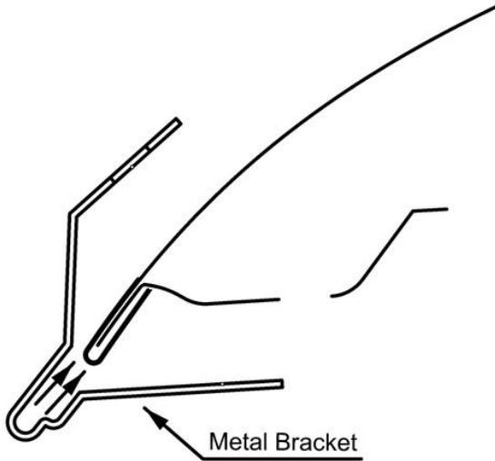
4. Install Metal Brackets over the hood edge in their correct positions. Align the hole in the bottom leg of the bracket with the round hole in the hood. See *Illustration*.
