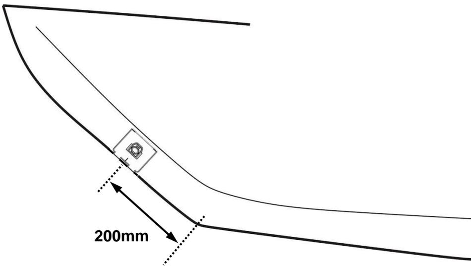
7. The positions of the pedestals are shown in **illustration**. Use the center mark on the leading edge of the pedestal for accurate measuring. The fingers incorporated on the leading edge of the pedestal will help ensure the correct position relative to the hood edge. When correctly positioned the fingers should contact the leading edge of the hood.
