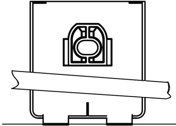
6. Dry fit the adhesive pedestals using masking tape to hold them in position.
