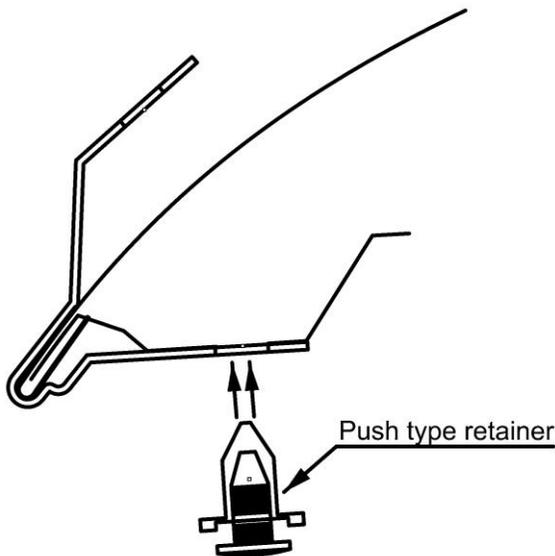
5. Insert a push type retainer through the metal bracket and into the hood. Ensure leg of the bracket is well seated against the surface of the hood and push the center pin of the retainer assembly to lock it into place. See *Illustration*.
