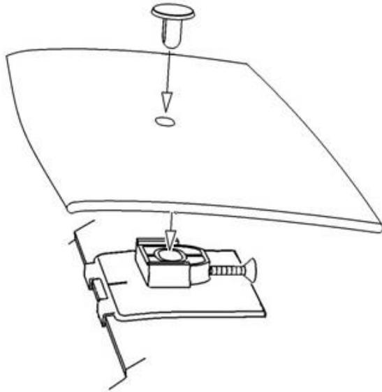
15. At the pedestal locations, drop a pin through the protector and into the pedestal.
