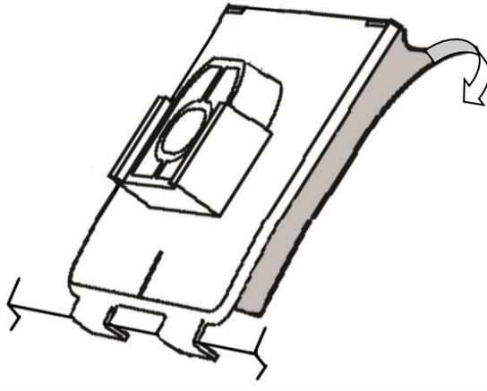
12. Remove the protective backing from the adhesive on the pedestals and install on the hood surface.
