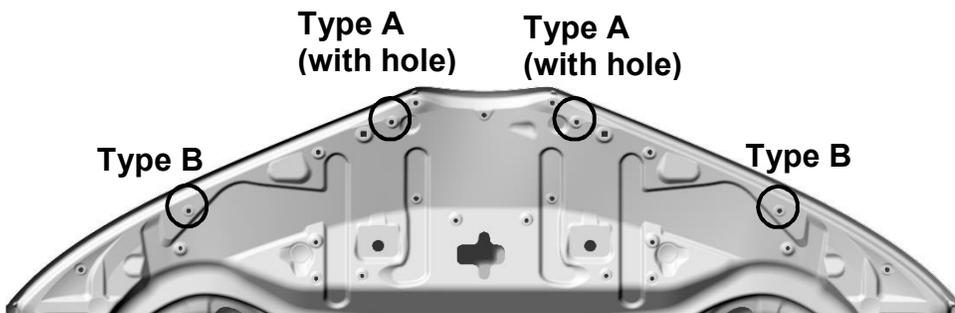
**NOTE: Use the Metal Bracket Guide to determine which brackets go in the proper locations.**
