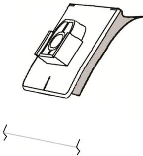
10. Remove the red protective backing from the pedestals using caution to avoid contaminating adhesive surface.
