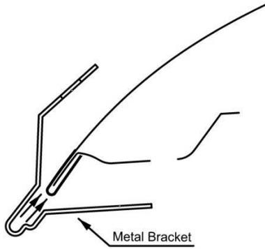
4. Install the four metal brackets on the hood edge over the anti-abrasion pads. Align the hole in the bottom leg of the bracket with the round hole in the hood. See *Illustration*.
