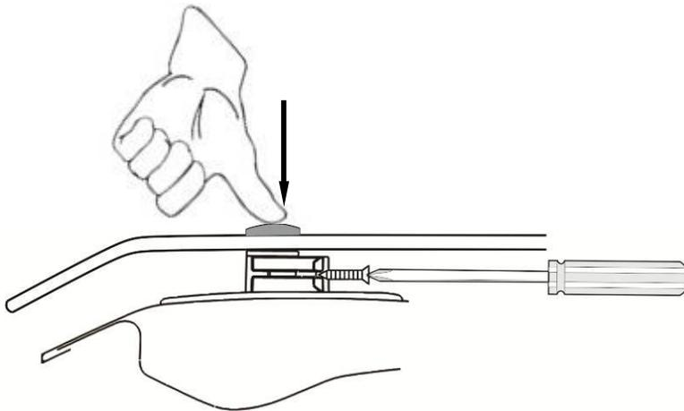
14. On some vehicles it may be necessary to adjust the hood bumpers and/or latch for proper clearance.
