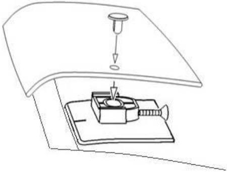
13. Insert a pin through the protector and into each of the two (2) pedestals. Maintain pressure on the head of the pin to ensure the protector is seated against the pedestal and tighten the screw until snug. Do not over-tighten!
