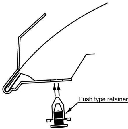
**NOTE:** Engaging the center pin of the push-type retainer is best accomplished by placing a #2 Philips drive screwdriver into the recess of the center pin and pushing the **pin followed by tightening 90 degrees to fully engage the retainer into the hood**. The retainer can be removed by unthreading the center pin with a Philips screwdriver, however initial installation is best done using the push-method described above.
