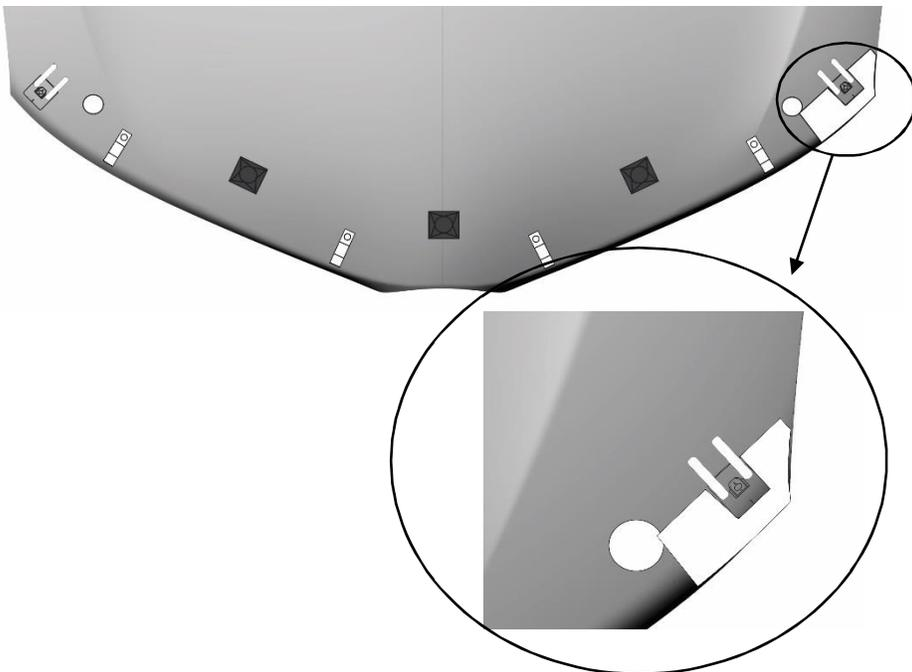
6. Test fit the adhesive pedestals using the supplied tape strips or masking tape to temporarily hold them in position.
