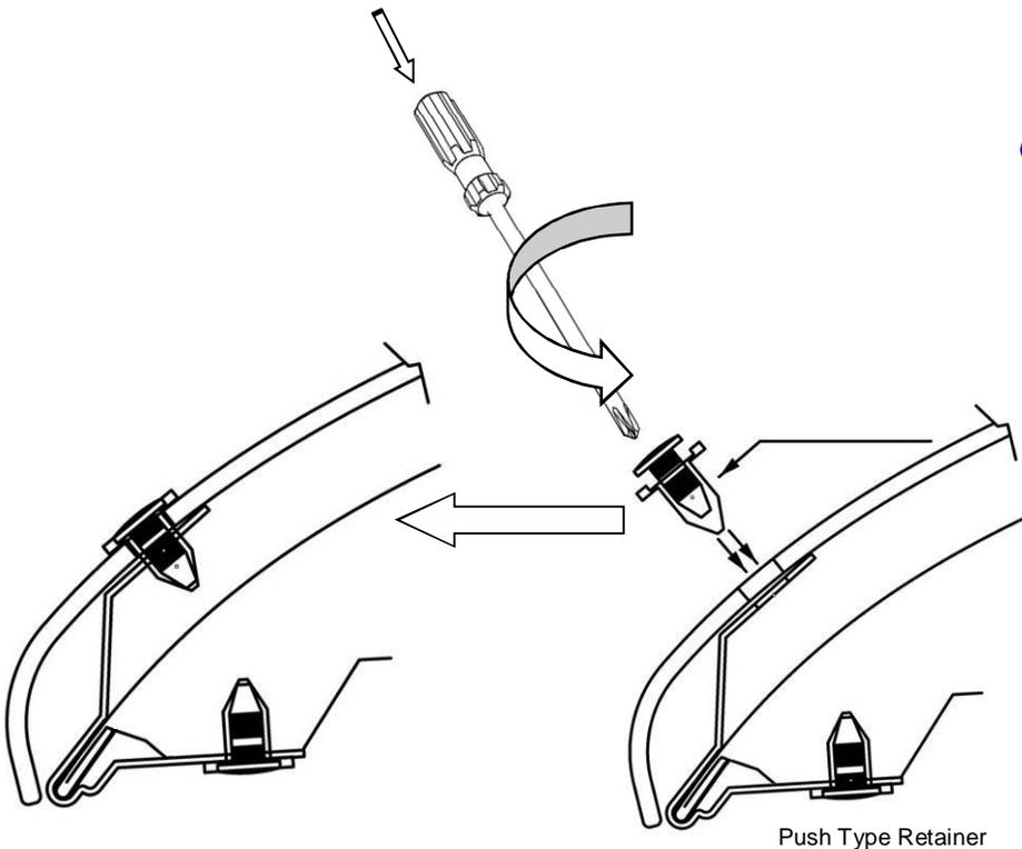
12. Place the protector on the hardware mounted to the hood and align the four (4) holes in the protector with the holes in the metal brackets.
