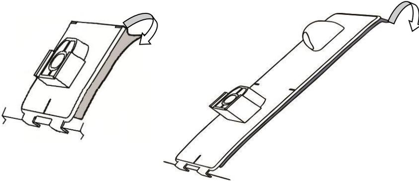
9. Remove the protective backing from the adhesive on the pedestals
