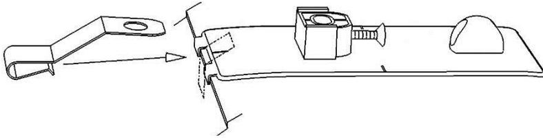
14. For the large adhesive pedestals over the grill, push a large metal mounting bracket over the hood edge and ensure the bracket is fully engaged
