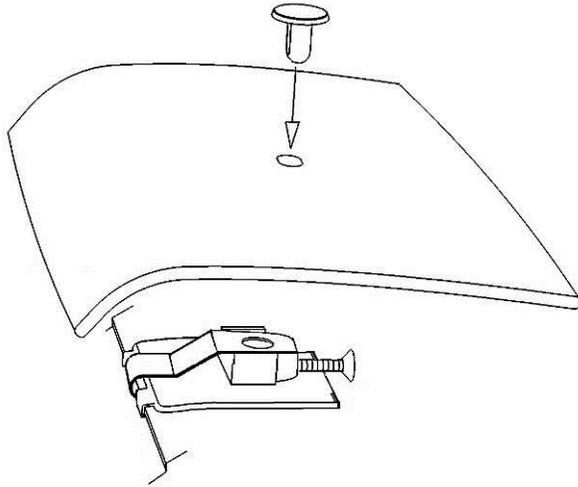
18. At the four (4) small pedestals, drop a pin through the protector and into the pedestal.
