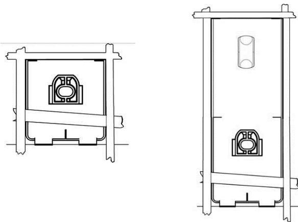
7. Remove the hood protector, and outline the perimeter of the pedestals with masking tape or the repositionable tape strips.
