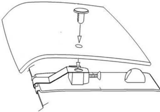
16. At the three (3) large pedestal locations drop a pin through the protector and into the pedestal
