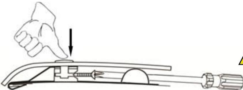
17. Maintain slight pressure on the pin, to ensure proper seating of the components, while simultaneously tightening the screw.
