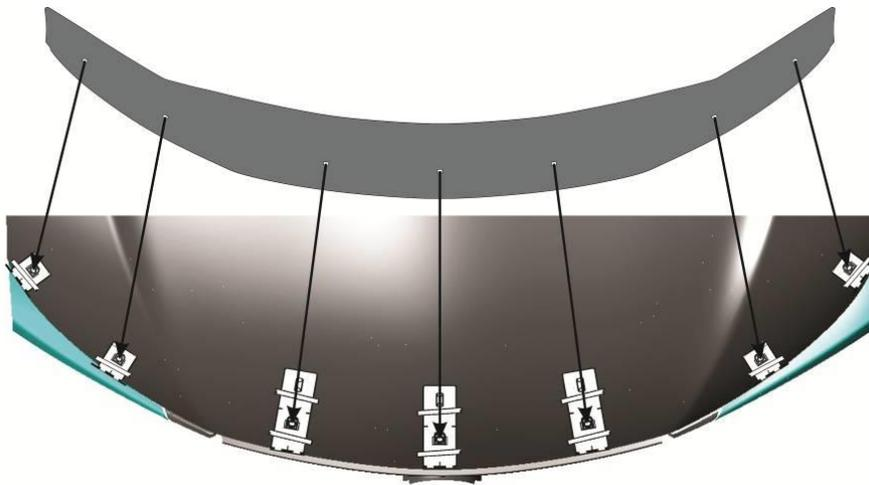
6. Place the hood protector on the pedestals to confirm proper positioning, make any necessary adjustments.
