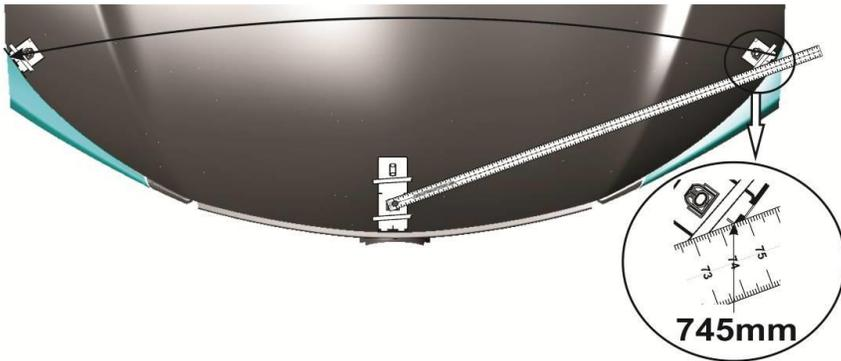
5. Use the center mark on the leading edge of the pedestals for accurate measuring.
