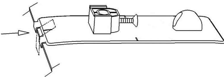
13. Peel and fold the small anti abrasion film pad in half over the hood edge between the fingers on the pedestal.
