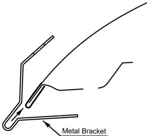
4. Install Metal Brackets over the hood edge in their correct positions. Align the hole in the bottom leg of the bracket with the round hole in the hood. *See Illustration.*
