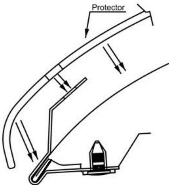
9. Place the protector temporarily onto the metal brackets aligning the holes in the protector with the holes in the metal brackets. This step will allow you to confirm the position of the adhesive pedestals.
