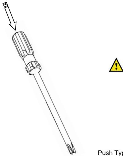
15. Place the hood protector on the hood resting on the two (2) metal brackets; align the 2 center holes in the protector with the holes in the metal brackets. Insert a “push type retainer” through the hole in the protector, and into the bracket. Ensure the protector is well seated against the surface of the metal bracket, and push the center pin of the retainer assembly to lock it into place.
