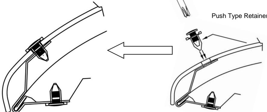
**NOTE:** Engaging the center pin of the “push type retainer” is best accomplished by placing a #2 Philips drive screwdriver into the recess of the center pin. Use a light force or tap on the end of the screwdriver to seat the pin into the retainer. The retainer can be removed by unthreading the center pin in the conventional manner with a Philips screwdriver, however initial or subsequent placement is best performed using the “push” method described above.
