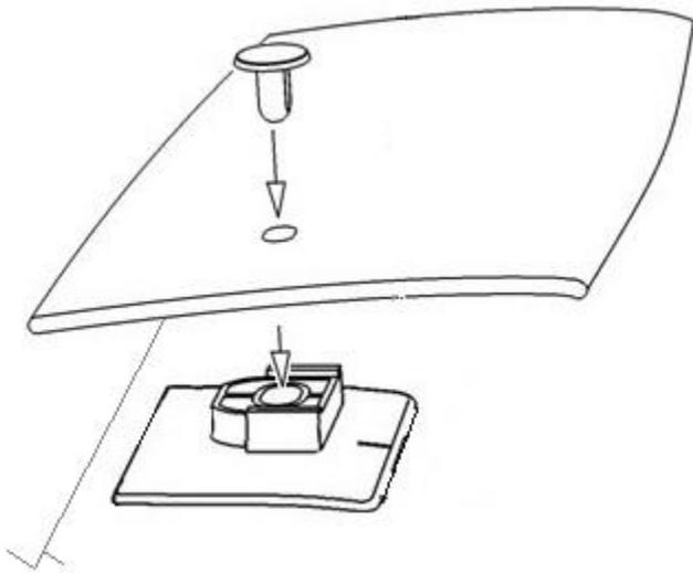
16. At the pedestal locations, drop a pin through the protector and into the pedestal.
