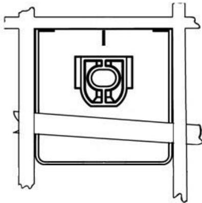
11. Remove the hood protector, and outline the perimeter of the pedestals with masking tape or the repositionable tape strips supplied to help final installation.
