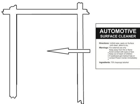
12. Remove the pedestals and thoroughly clean the outlined area with the alcohol wiping pad. Dry with a soft cloth or paper towel. This will insure all wax, finger prints and oils are removed from the hood surface in the bonding area.
