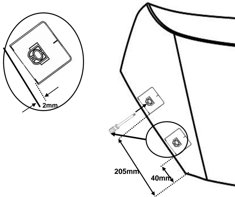
8. The positions of the pedestals are shown in **illustration**. Use the corner of the pedestal for the measurements. The pedestals should have an even 2mm gap from the edge of the hood to the bottom edge of the pedestal
