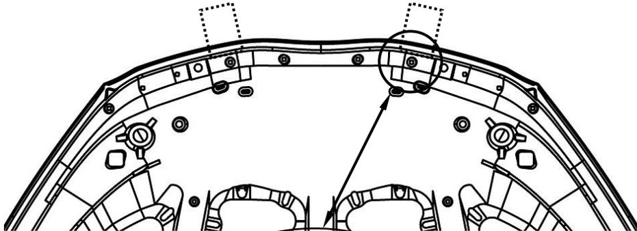
Open the hood of the vehicle. Peel and fold anti-abrasion film pads in half over the edge of the hood, in the two (2) locations shown.
