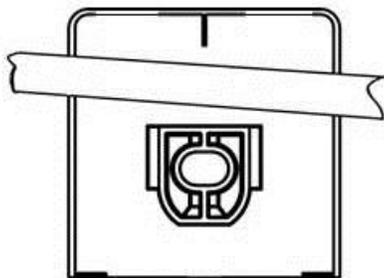
7. Dry fit the adhesive pedestals using masking tape or the repositionable tape strips supplied to hold them in position.
