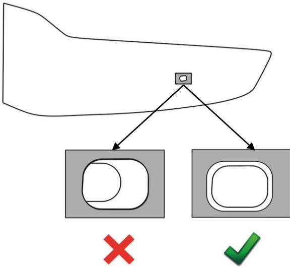
10. Confirm correct positioning of the pedestals, by adjusting the pedestal position on the hood to align with the holes in the hood protector.
