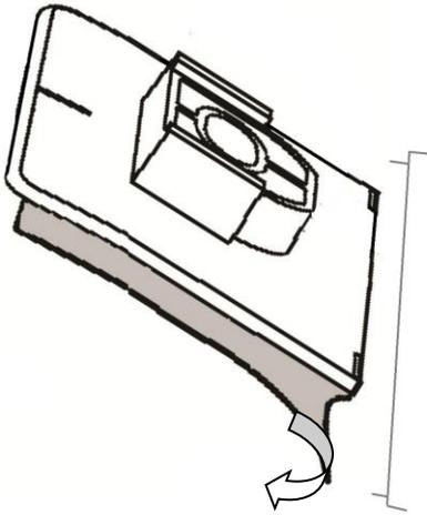
13. Remove the protective backing from the adhesive on the pedestals and install on the hood surface.
