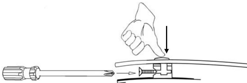
18. On some vehicles it may be necessary to adjust the hood bumpers and/or latch for proper clearance.
