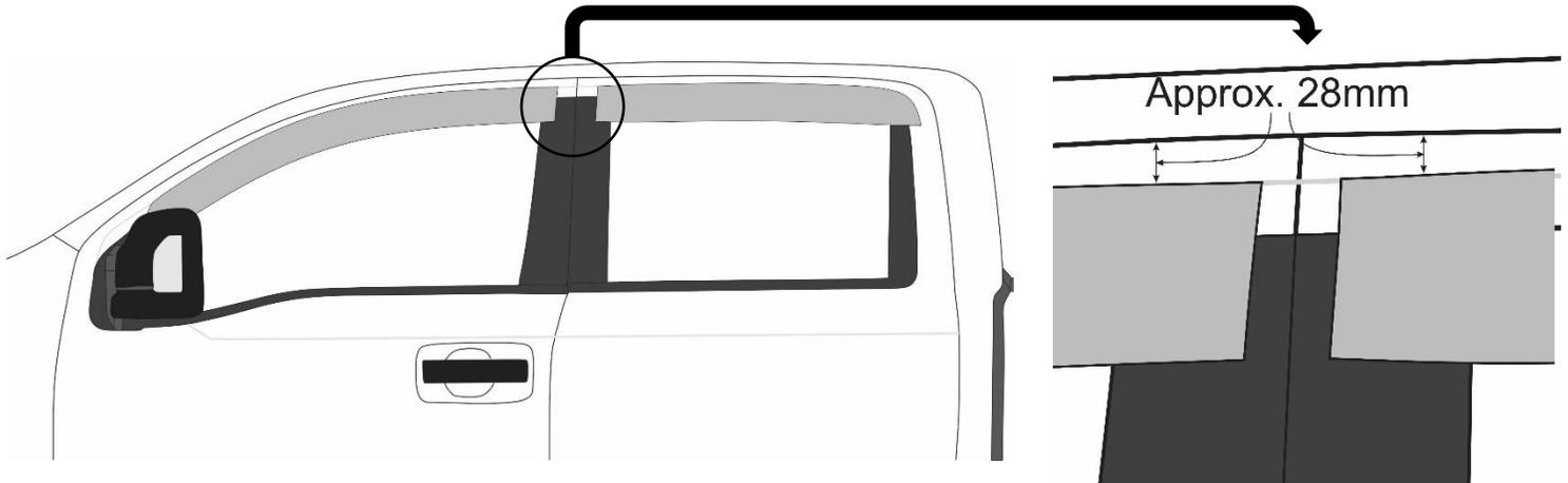
5. Clean the mounting areas aggressively with alcohol wiping pad and dry with a clean cloth or paper towel to remove any finger prints, oils or waxes that may be on the surface
