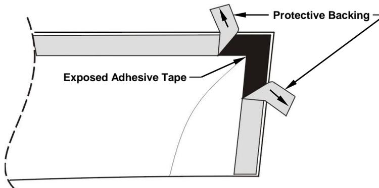
7. Reposition the deflector on the window frame as described in steps #2 and #3. Adjust the deflector for best fit. While pressing the deflector into place, pull the protective backing out from between the deflector and door frame without disturbing the fit of the deflector.
