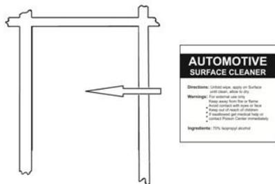
6. Remove the pedestals and thoroughly clean the outlined area with the alcohol wiping pad. This will insure all wax, finger prints and oils are removed from the hood surface in the bonding area.
