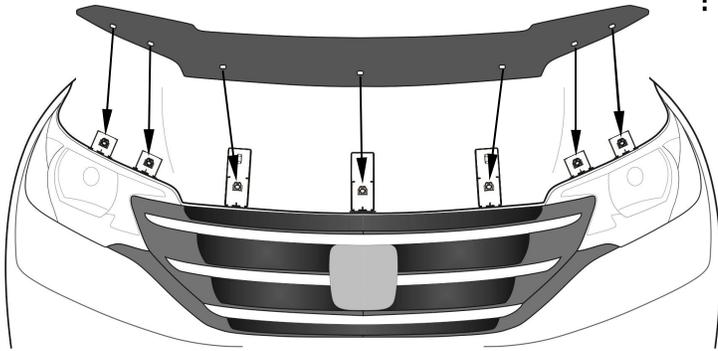
4. Place the hood protector on the pedestals to confirm proper positioning. Ensure the holes in the protector align with those in the pedestals and confirm the deflector is centered on the hood by measuring the overhang of the protector at both sides of the hood. The measurement should be the same on both sides +/- 2mm. If necessary, reposition the pedestals so all attachment positions are correct and the protector is well centered.
