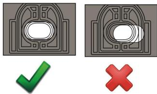
5. Remove the hood protector, and outline the perimeter of the pedestals with masking tape or the repositionable tape strips supplied to help final installation.
