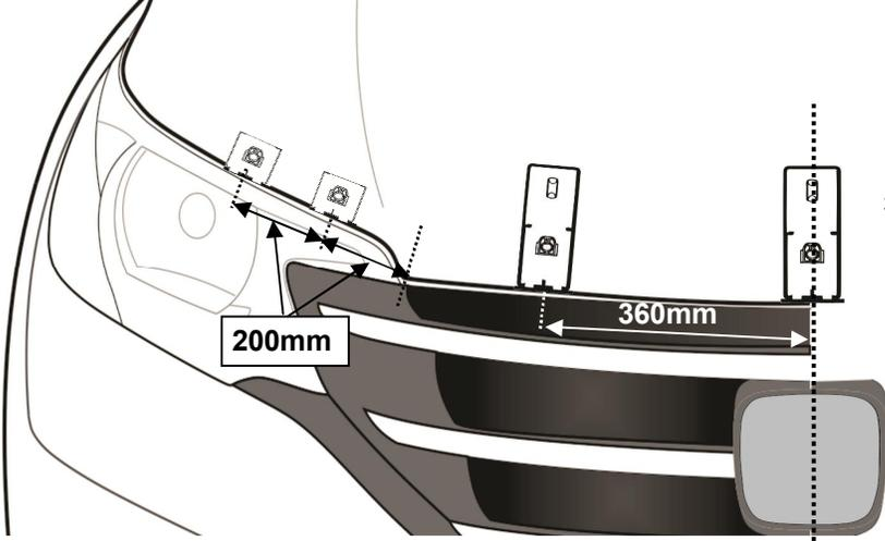
3. The positions of the pedestals are shown in **illustration**. Use the center mark on the leading edge of the pedestals for accurate measuring. The fingers incorporated on the leading edge of the pedestal will help ensure the correct position relative to the hood edge. When correctly positioned the fingers should contact the leading edge of the hood.
