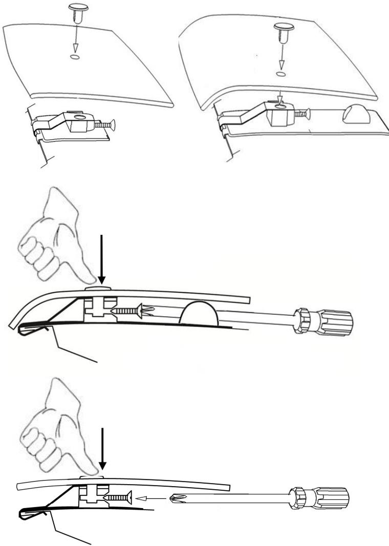
11. Place the hood protector on the pedestals and drop a pin through the protector and into the pedestal. Maintain slight pressure on the pin, to ensure proper seating of the components, while simultaneously tightening the screw. Repeat for remaining pedestal locations.
