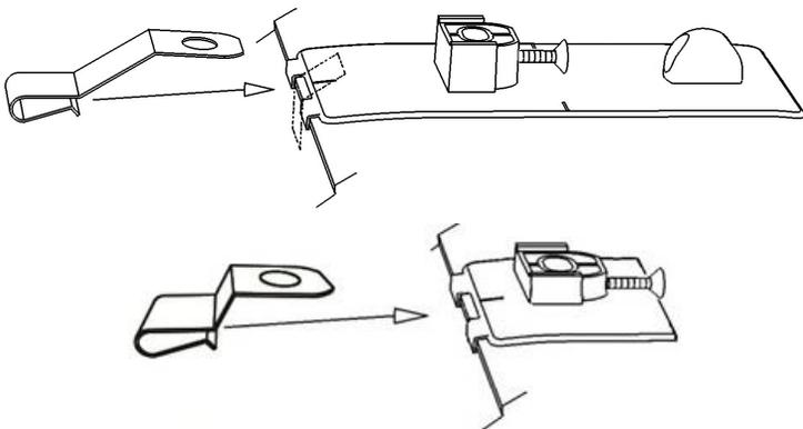
10. Push a metal mounting bracket over the hood edge on top of the anti-abrasion pad installed previously. Ensure the bracket is fully engaged over the hood edge and the hole in the bracket is aligned with the hole in the pedestal.
