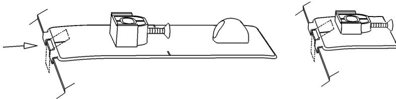
9. Peel and fold the anti-abrasion film pad in half over the hood edge between the fingers on the pedestal.
