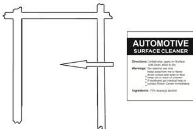
3. The positions of the pedestals are shown in **illustration**. Use the center mark on the leading edge of the pedestals for accurate measuring. The fingers incorporated on the leading edge of the pedestal will help ensure the correct position relative to the hood edge. When correctly positioned the fingers should contact the leading edge of the hood.
