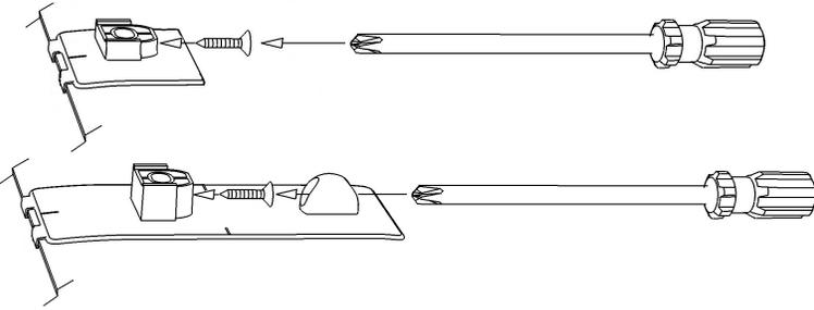
8. Start a #6 x 5/8 flat head screw into each pedestal a few turns. The tip of the screw must not protrude into the hole where the attachment pin will install later.
