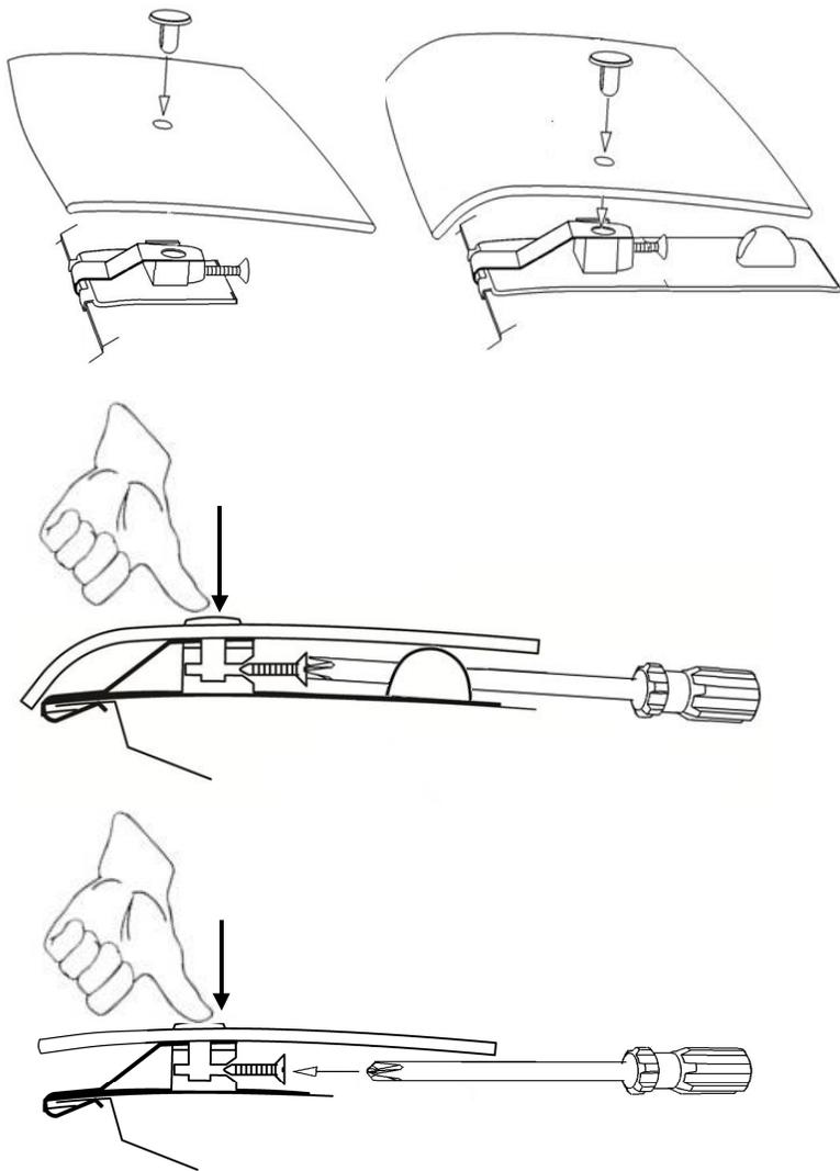
11. Place the protector on the pedestals and drop a pin through the protector and into the pedestal. Maintain slight pressure on the pin, to ensure proper seating of the components, while simultaneously tightening the screw. Repeat for remaining pedestal locations.
