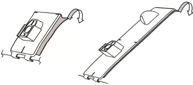
7. Remove the protective backing from the adhesive on the pedestals and install on the hood surface.
