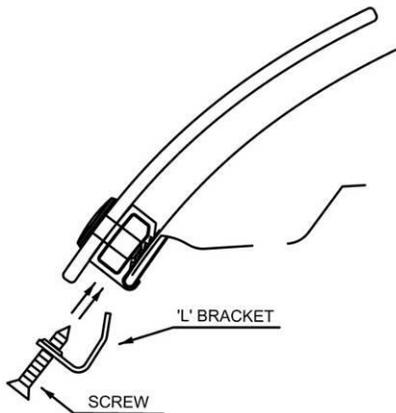
11. Start a screw through an L bracket and into the clip a few turns.
