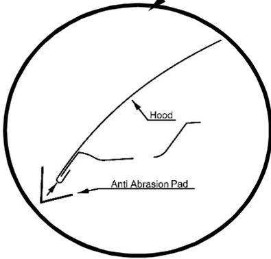
4. Install the three metal brackets on the hood edge over the anti-abrasion pads. Align the hole in the bottom leg of the bracket with the round hole in the hood. See illustration.
