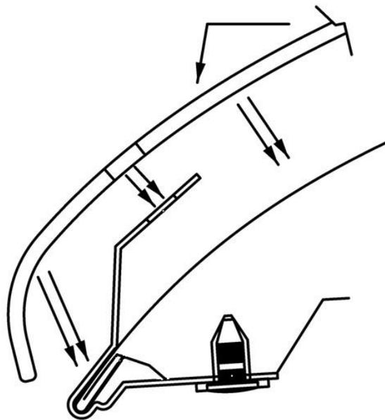
6. Place the hood protector on the hood, resting on the three metal brackets.
