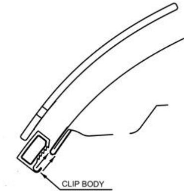
9. Place a clip body over one of the anti-abrasion pads on the edge of the hood.
