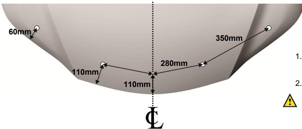
3. Open the hood of the vehicle. Peel and fold the anti-abrasion pads in half over the edge of the hood, in line with the 3(three) holes under the hood, as shown. See illustration.
