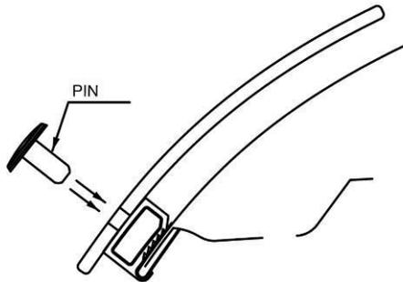
10. Insert a pin through the protector and into the clip.
