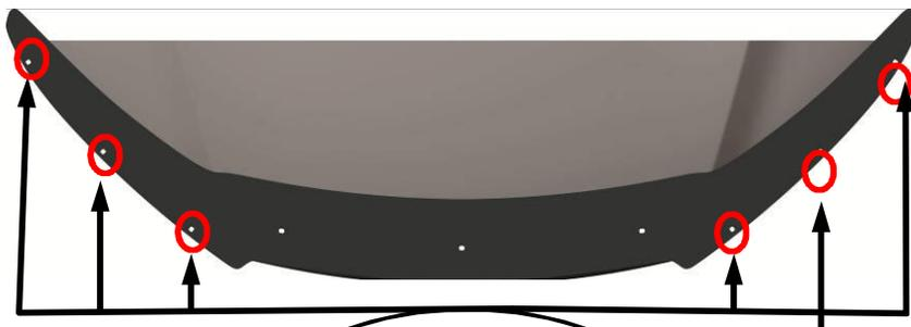
8. Peel and fold the anti-abrasion pads in half over the edge of the hood in line with the three holes in the protector over each of the headlights. See *Illustration*. Repeat for remaining push-type retainers.
