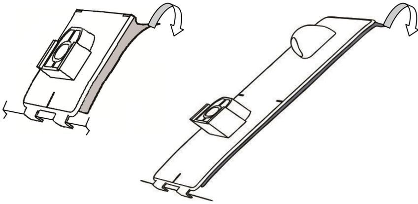
10. Remove the protective backing from the adhesive on the pedestals and install on the hood surface.
