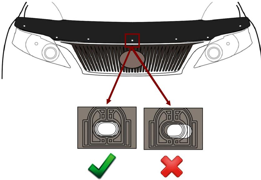
7. Confirm correct positioning of the pedestals, by adjusting the pedestal position on the hood to align with the holes in the hood protector.
