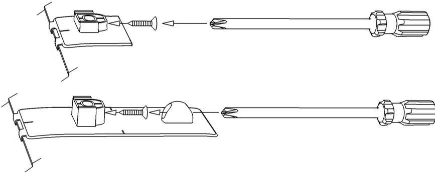
11. Start a #6 x 5/8 flat head screw into each pedestal a few turns. The tip of the screw must not protrude into the hole where the attachment pin will install later.
