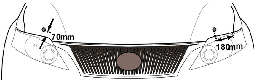
3. Install the two (2) bumpons as shown. **Attention: Bumpons must be installed on the hood, not on the deflector!!!** If the bumpons are installed on the deflector, they may wear through the paint.
