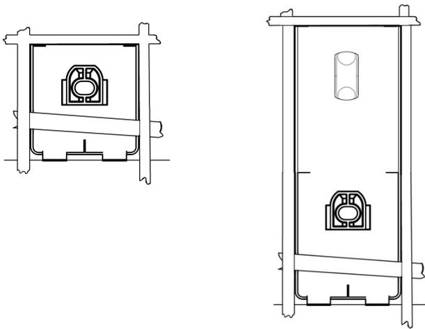
8. Remove the hood protector, and outline the perimeter of the pedestals with masking tape or the repositionable tape strips supplied to help final installation.
