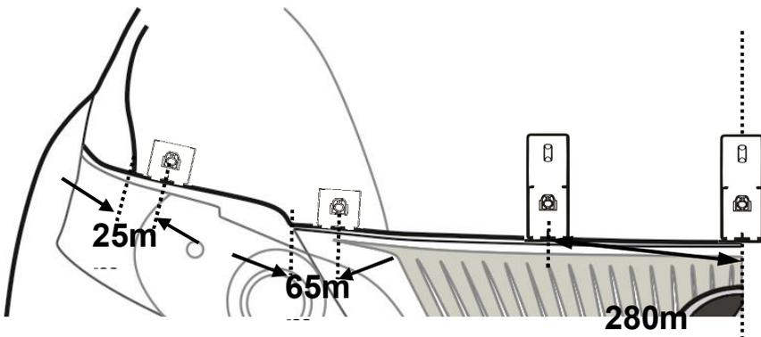
4. Dry fit the adhesive pedestals using masking tape or the repositionable tape strips supplied to hold them in position.
