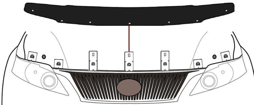
6. Place the protector temporarily onto the Adhesive pedestals, aligning the holes in the protector with the holes in the pedestals. This step will allow you to confirm the position of the adhesive pedestals.
