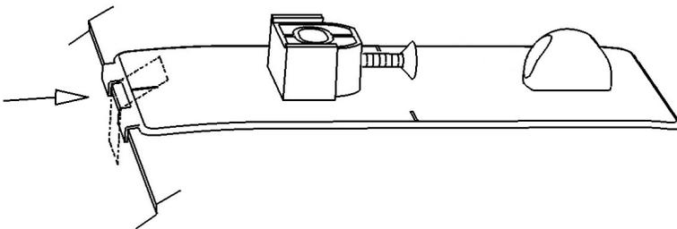
13. Push a metal mounting bracket over the hood edge on top of the anti abrasion pad installed previously. Ensure the bracket is fully engaged over the hood edge and the hole in the bracket is aligned with the hole in the pedestal.
