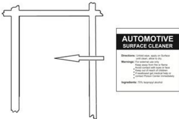
9. Remove the pedestals and thoroughly clean the outlined area with the alcohol wiping pad. Dry with a clean cloth or paper towel. This will insure all wax, finger prints and oils are removed from the hood surface in the bonding area.
