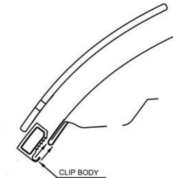
17. Place a clip over each of the anti-abrasion film pads on the edge of the hood.
