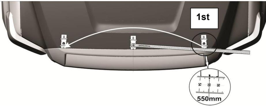
6. Use the center mark on the leading edge of the pedestals for accurate measuring.
