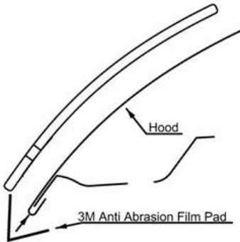
16. Peel and fold two (2) of the anti-abrasion film pads in half over the hood edge aligned with the inner holes of the protector in the area above the headlights.
