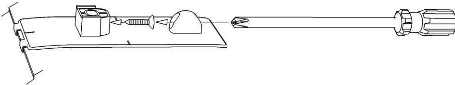
13. Start a screw into each pedestal a few turns. The tip of the screw must not protrude into the hole where the attachment pin will install later.
