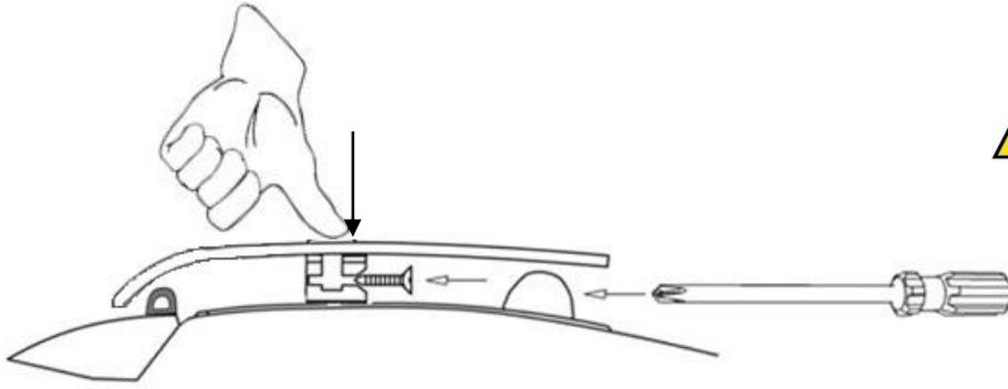
15. To ensure proper seating of the components, maintain slight pressure on the pin while simultaneously tightening the screw.
