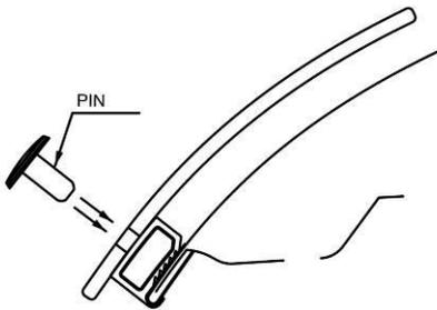
18. Insert a pin through the protector into each of the clips.
