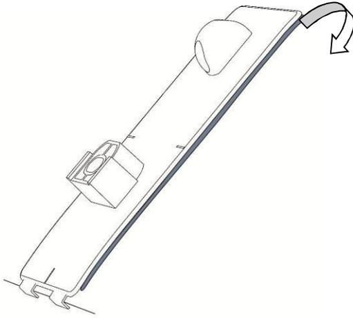
11. Remove the protective backing from the adhesive on the pedestals
