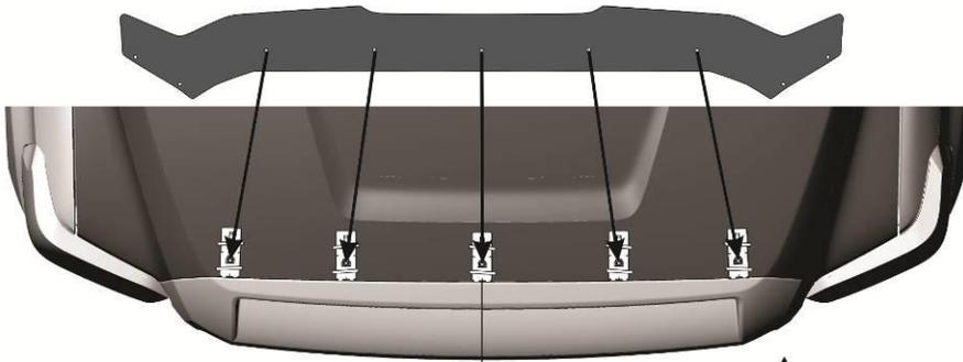
7. Place the hood deflector on the pedestals to confirm proper positioning, make any necessary adjustments.
