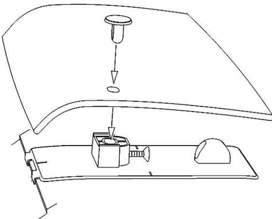
14. At the pedestal locations, drop a pin through the protector and into the pedestal.
