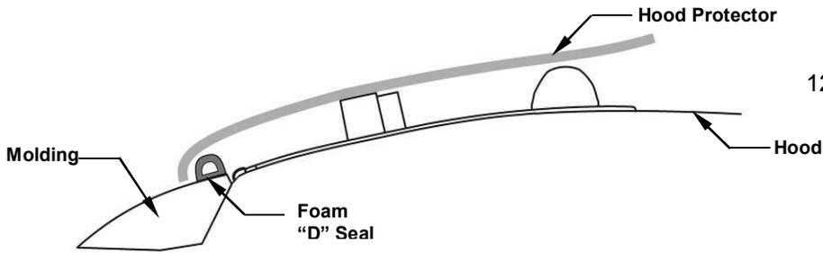
12. Install the Foam "D" seal as shown in the illustrations. It may be necessary to trim the Foam "D" seal to the correct length. Refer to illustration in step #10
