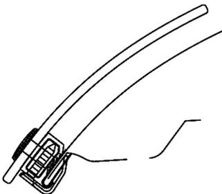
13. Peel and fold the two (2) large anti-abrasion pads in half over the hood edge aligned with the holes of the protector in the area above the headlights.
