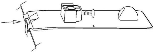
10. Peel and fold the small anti-abrasion pads in half over the hood edge between the fingers on each of the pedestals.
