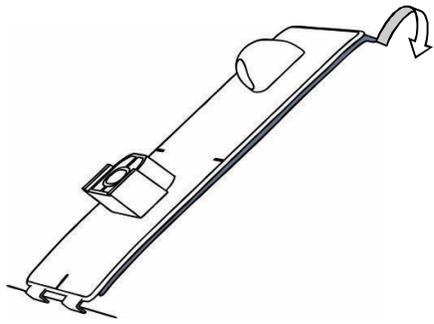
8. One pedestal at a time, remove the protective backing from the adhesive and install on the hood surface.
