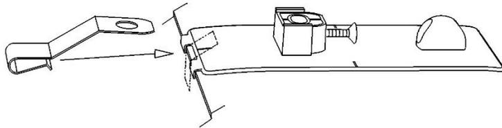
11. Push metal mounting brackets over the hood edge aligned with the anti abrasion pads installed previously. Ensure the bracket is fully engaged over the hood edge and the hole in the bracket is aligned with the hole in the pedestal.
