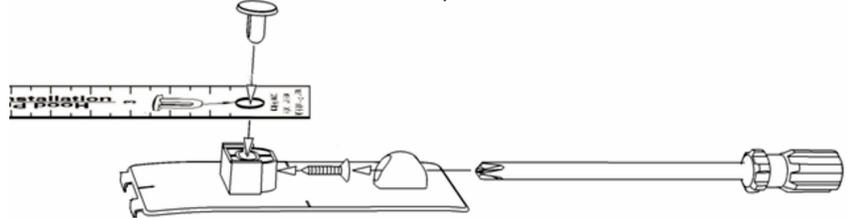
**Locate center pedestal using installation tape measure and/or supplied centering template.**
