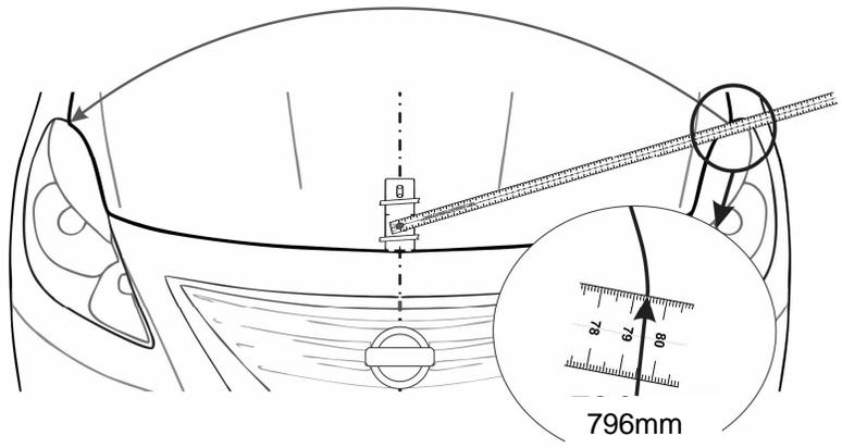
⚠ **\*Tape measure is always located below measuring point.**
