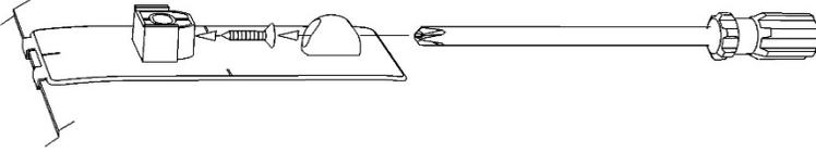
9. Start a screw into each pedestal a few turns. The tip of the screw must not protrude into the hole where the attachment pin will install later.
