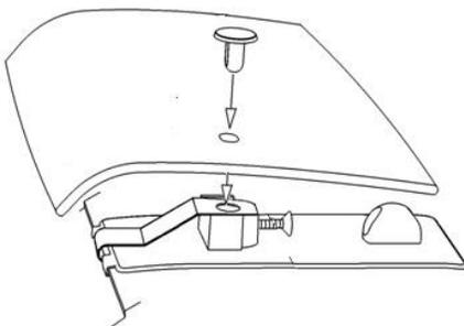
12. Place the protector on the pedestals and starting at the center position install a pin through the protector and into the pedestal. Maintain slight pressure on the pin to ensure proper seating of the components, while simultaneously tightening the screw a few turns. Repeat for remaining pedestal locations.
