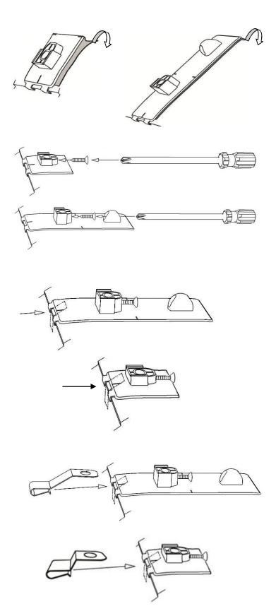
One pedestal at a time, remove the protective backing from the adhesive and install on the hood surface.
