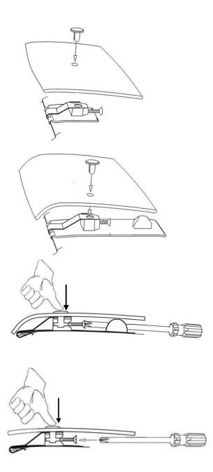
12. Place the protector on the pedestals, and starting at the center location install a pin through the protector and into the pedestal. Maintain slight pressure on the pin to ensure proper seating of the components, while simultaneously tightening the screw a few turns. Repeat for remaining pedestal locations.
