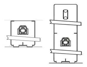
The positions of the pedestals are shown in the **illustrations**. Use the center mark on the leading edge of the pedestals for accurate measuring. The fingers incorporated on the leading edge of the pedestal will help ensure the correct position relative to the hood edge. When correctly positioned the fingers should contact the leading edge of the hood.
