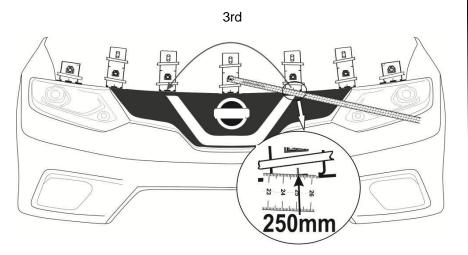
Starting at the outer most locations dry fit the remaining pedestals, as shown, using masking tape or re-usable tape strips supplied to temporarily hold them in position.
